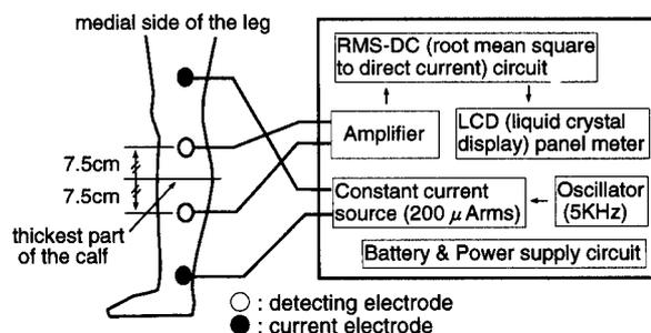
Fig. 1. Block diagram of the apparatus and the electrode location.
