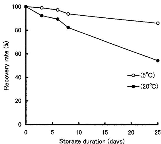
**Fig. 1.** Effect of the storage stability condition of the sampling tube at room temperature (20°C) and in a refrigerator (5°C).
