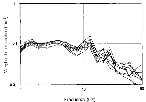
**Fig. 2.** Spectral analysis of the vertical vibration measured on the seat pans of 12 taxis.
