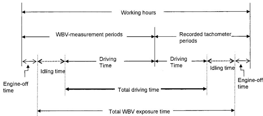
Fig. 1. Structure for measuring time.
