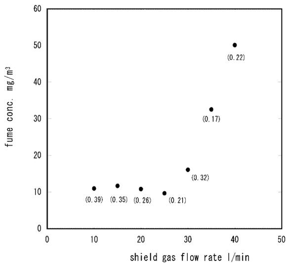
**Fig. 3.** The effect of the shielding gas flow rate on the fume concentration at the assumptive breathing zone. The plots are the arithmetic means of 10 measurements, and the RSD of each plot is shown in the parentheses. The work piece settings were layout ①.
