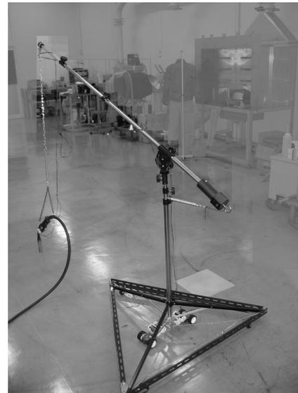
**Fig. 4.** Example of a suspending unit for a fume-exhaust gun.
