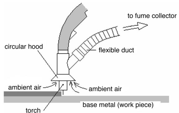
Fig. 1. Fume exhaustion by means of a fume-exhaust gun.
