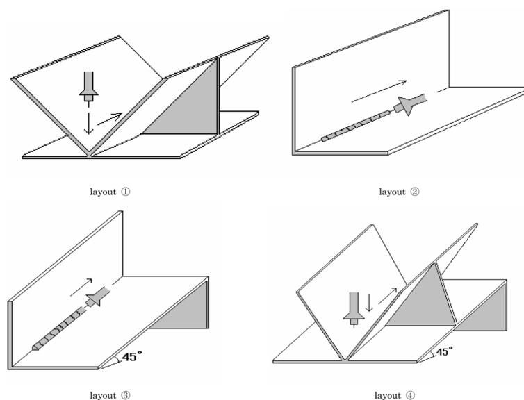
Fig. 2. Layouts of the base metals (work pieces).
