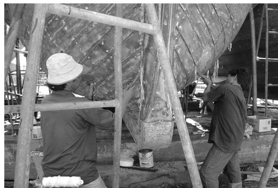
Fig. 2. Pulling out decayed caulking material and re-caulking with lead-mingled yarn.
