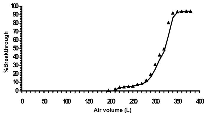
**Fig. 4.** Breakthrough curve of 200 ppb 4-vinyl-1-cyclohexene in dry air adsorbed on 100 mg of charcoal at a flow rate of 0.5 l/min when using 1.0 ml of effluent air injected into the gas chromatograph.
