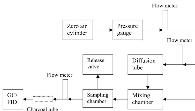
**Fig. 1.** Schematic diagram of instrumentation required for 4-vinyl-1-cyclohexene generation, capture and analysis.
