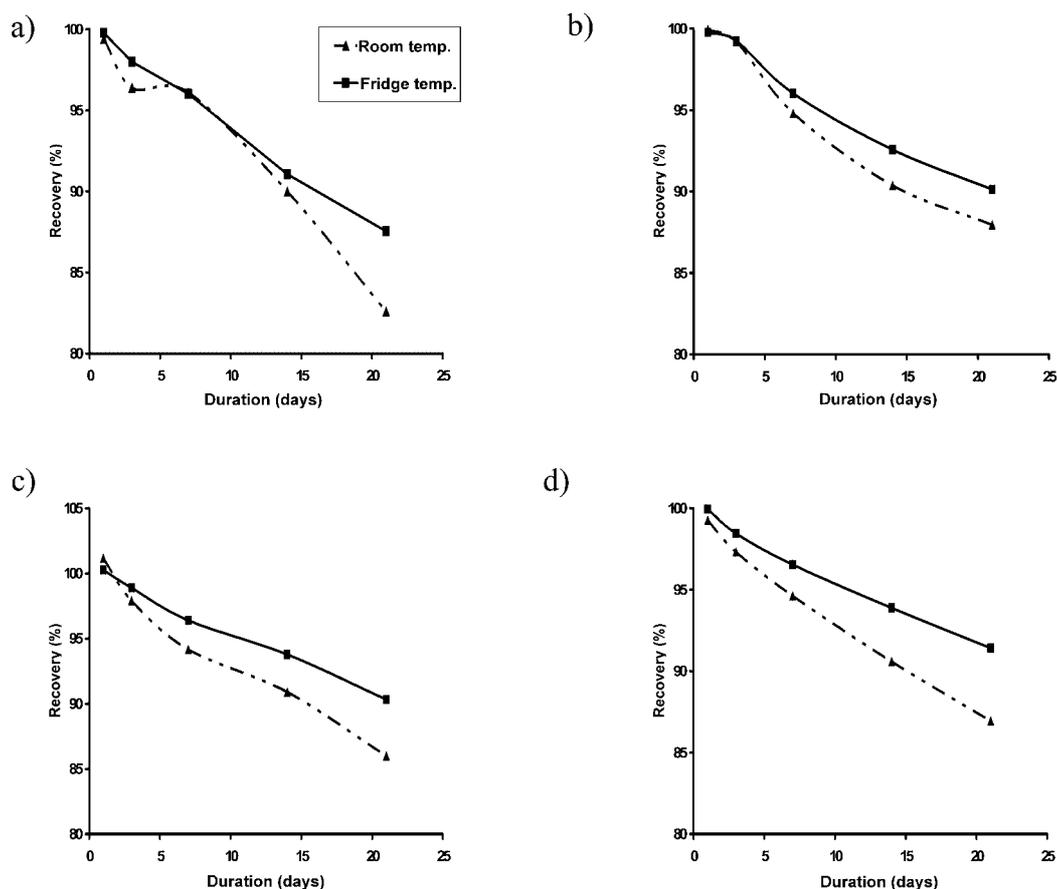
**Fig. 5.** Storage stability of four loading levels of spiked 4-vinyl-1-cyclohexene on charcoal tube at room and refrigerated temperatures: a) 0.412  $\mu\text{g}$  4-vinyl-1-cyclohexene, b) 2.062  $\mu\text{g}$  4-vinyl-1-cyclohexene, c) 4.125  $\mu\text{g}$  4-vinyl-1-cyclohexene, and d) 8.250  $\mu\text{g}$  4-vinyl-1-cyclohexene.
