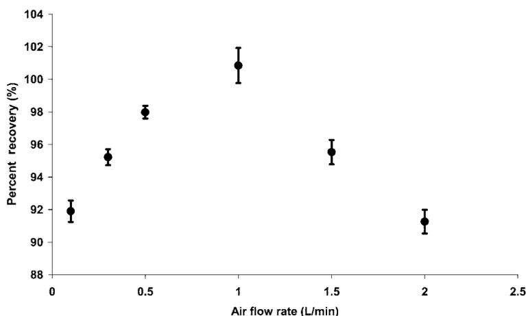
**Fig. 3.** Percent recoveries of 4-vinyl-1-cyclohexene from charcoal tubes after sampling of 200 ppb 4-vinyl-1-cyclohexene vapor in 100 l air at flow rates of 0.1, 0.3, 0.5, 1.0, 1.5 and 2 l/min.
