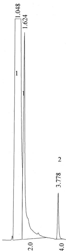
**Fig. 2.** Chromatogram of standard 4-vinyl-1-cyclohexene in carbon disulfide: (1) carbon disulfide (2) 4-vinyl-1-cyclohexene.
