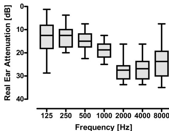
**Fig. 2.** Attenuation results for EM at each octave band in Real Ear Attenuation at Threshold test (n=20).
