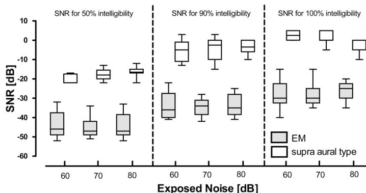
**Fig. 3.** SNR recorded for 50%, 90%, and 100% monosyllable intelligibility in 60–80 dB noise-exposed environment by type of communication device at speech audiometry (n=10).
