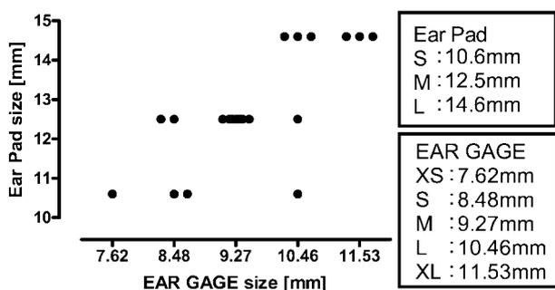
**Fig. 1.** Ear pad selection with respect to size of external ear canal measured by EAR-GAGE in Real Ear Attenuation at Threshold test (n=20).
