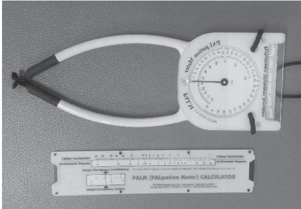
Fig. 1. Features of the palpation meter (PALM).
