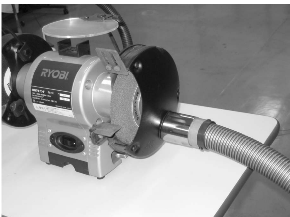
Fig. 1-3. Direct exhaustion from the grinding wheel shroud.
