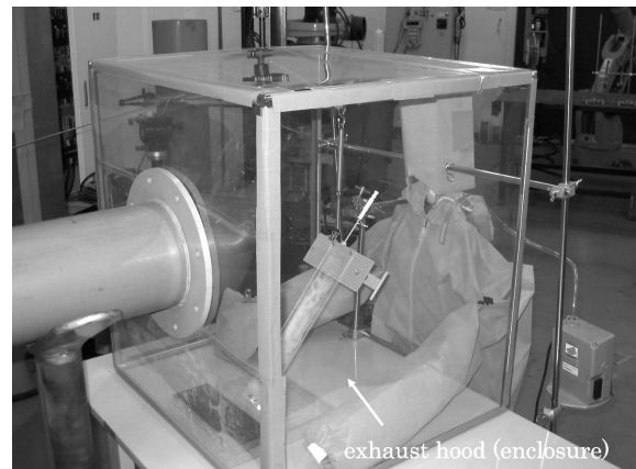
Fig. 3-3. Dummy worker and local exhaust ventilation hood (open face=60 × 55 cm) in this experiment.
